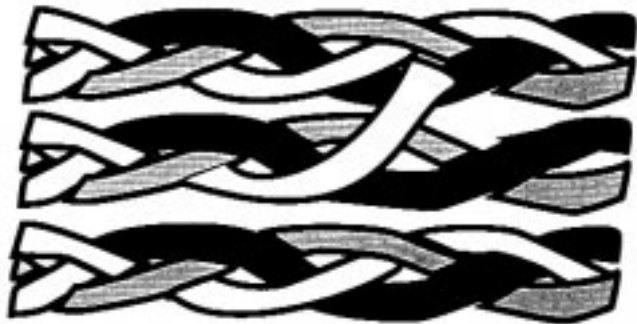
Figure 2 Fibers shown slightly separated with a cross link between two parallel fibers. This leads to decreased strength and inflexibility.
