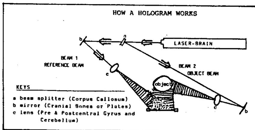
Since light travels in a wave pattern and since the angles of these two light sources meet at different angles an interference pattern is set up which allows the photographic plate to record the holographic three dimensional image. The image has both height, width, and most-important depth which in the case of holography is a parallex quality.
